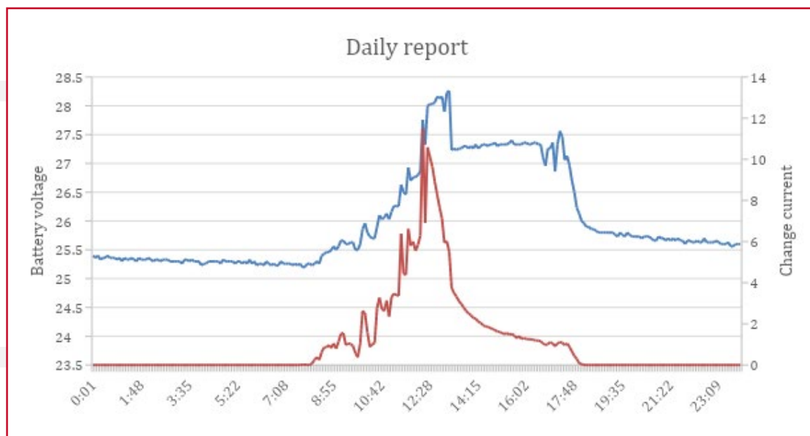
FIG.7 Daily trend of battery voltage (blue) and charging current due to the solar panel (red).
