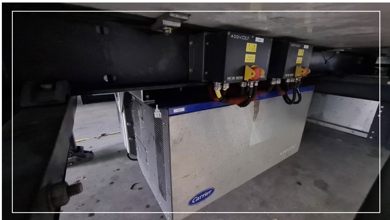
FIG.12 The ADDVOLT system is positioned under the trailer.
